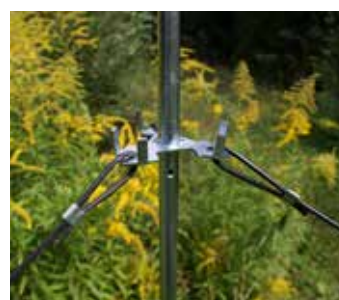
... mount the three bark beetle slit traps on the stand. Tip: Use pliers to bend and, thereby, slightly open hooks to facilitate installation.
