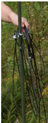
... place trap stand on it. Tighten the three guy ropes and use the pegs provided to secure stand to ground ...
