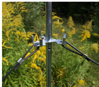
...Hook the three slot traps to the hooks.
