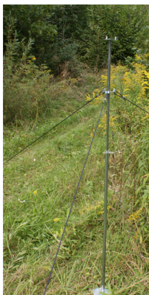
... place the three-trap stand on top. Next tension on the 3 tensioning ropes well and anchor to the ground using the supplied pegs...
