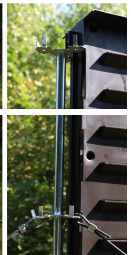
... mount the three bark beetle slit traps on the stand. Tip: Use pliers to bend and, thereby, slightly open hooks to facilitate installation.
