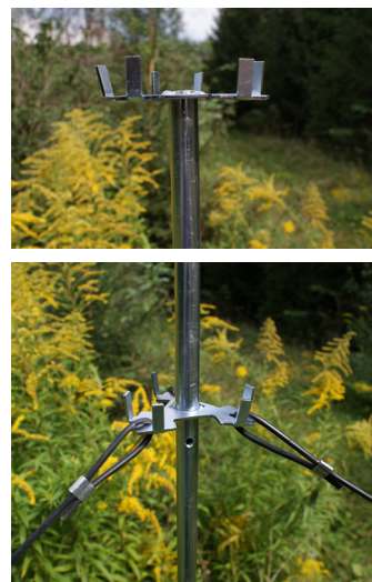
... mount the three bark beetle slit traps on the stand. Tip: Use pliers to bend and, thereby, slightly open hooks to facilitate installation.
