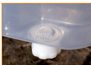
For wet trapping: Plug caps are installed.
