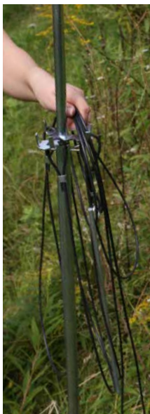
... place the three-trap stand on top. Next tension on the 3 tensioning ropes well and anchor to the ground using the supplied pegs...
