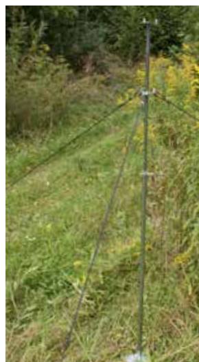
... place trap stand on it. Tighten the three guy ropes and use the pegs provided to secure stand to ground ...
